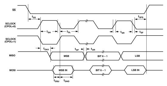
Figure 58. SPI Slave Mode Timing (CPHA = 1)
